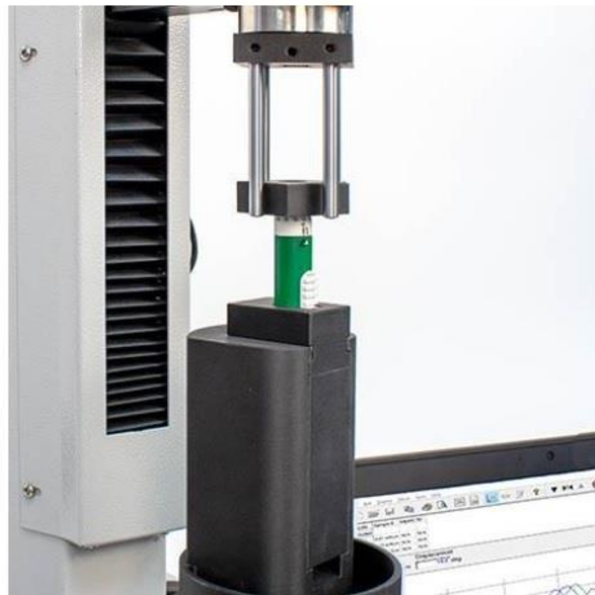
Dosage control dial torque testing with graphical results
